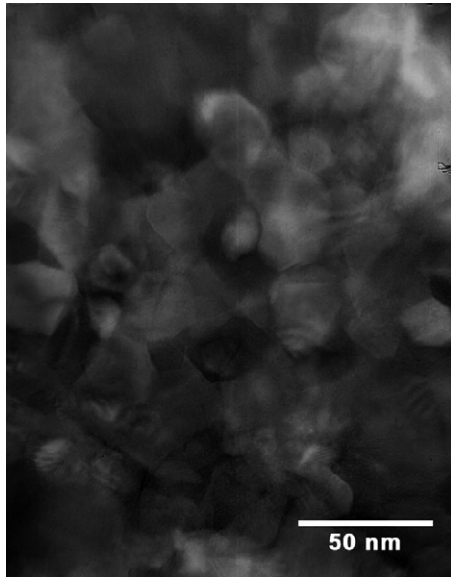
Fig. 5. TEM observation of powder (9.7 mol% \text{YO}_{1.5} ) obtained by sol-gel route.
